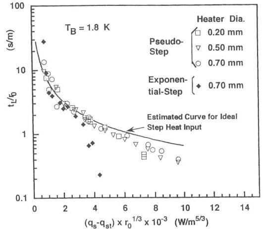
Fig.1 Relation between  $t_L/r_0$  and  $(q_s - q_{st})r_0^{1/3}$  for various diameter wires
