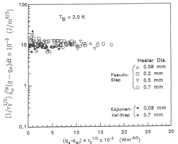
Fig.2 Integrated values of excess heat fluxes beyond  $q_{st}$  until the end of lifetime for various diameter wires
