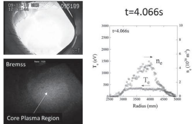
Fig. 1. A tangential view of a LHD plasma observed with a standard CCD camera (upper-left), an image of Bremsstrahlung observed with a fast framing camera (lower-left), and the radial profiles of electron temperature and density in a high density discharge.
