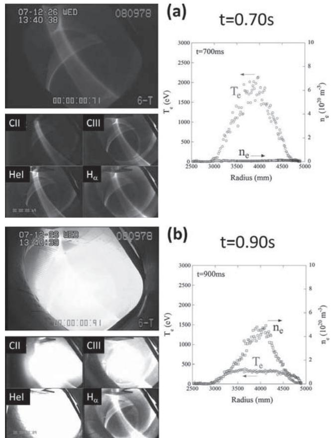
Fig. 2. Tangential plasma images observed with CII, CIII, HeI and  $H_\alpha$  interference filters before (a) and after (b) the formation of high density core plasma by pellet injections (lower-left). The other images/figures are same as those in Figure. 1.
