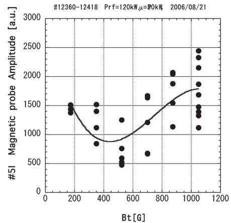
Fig.3 Wave magnetic fields measured by magnetic probe (#51) versus Bt.
