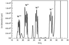
Fig. 2. Mass spectrum in introducing W(CO)<sub>6</sub>.
