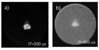
Fig.2 Images of IR camera for tungsten samples with a) a sandblasted surface and b) a mirror surface. Surface temperatures and the integrated times are  $277^{\circ}$ C and  $200 \,\mu$ s for a), and  $272^{\circ}$ C and  $800 \,\mu$ s for b) respectively.
