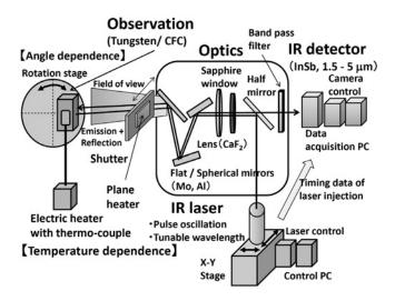
Fig. 1 Conceptual diagram of proof-of-principle experiment for in-situ calibration technique of infrared camera measurement
