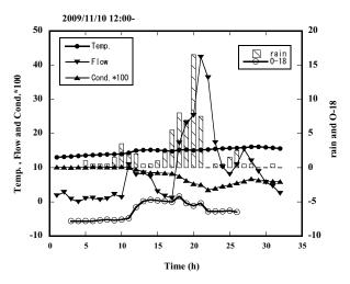
Fig.2 Variation of temperature, flow rate, conductivity, rainfall and O-18 ratio in river water at one rain event
