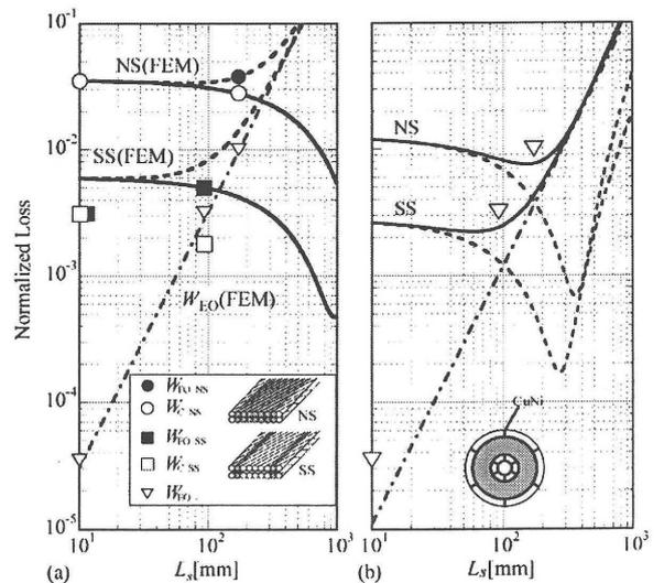
Fig. 1 Dependence of coupling losses on strand twist pitch.
