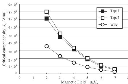
Fig.1 Critical current densities of the twisted MgB<sub>2</sub> multifilamentary round wire and tapes.
