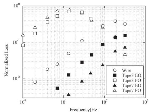
Fig. 2 Frequency dependences of coupling losses in the twisted MgB<sub>2</sub> multifilamentary wire and tapes.
