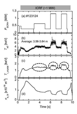
Figure 1. The typical time evolution of (a)  $P_{\rm ECRH}$ , (b)  $T_{\rm e0}$ , (c)  $T_{\rm i\_crystal}$  and (d)  $n_{\rm e\_fir}$ . The plasma was sustained using 0.27 MW ECRH and ~1 MW ICRF and the additional ECRHs were superimposed during 3-5 s (0.37 MW), 6-7 s (1 MW) and 8-9 s (1 MW).
