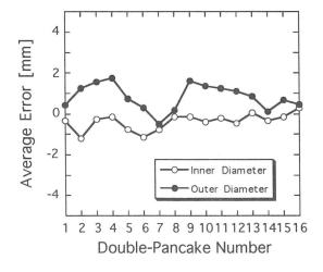
Fig. 2. Average manufacturing errors of the double-pancakes for the OV coils
