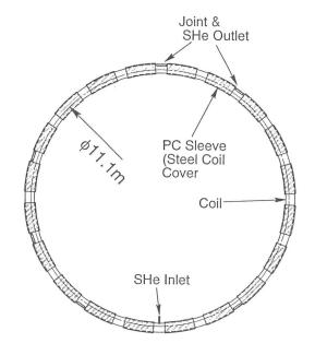
Fig. 1. Top View of the OV coil
