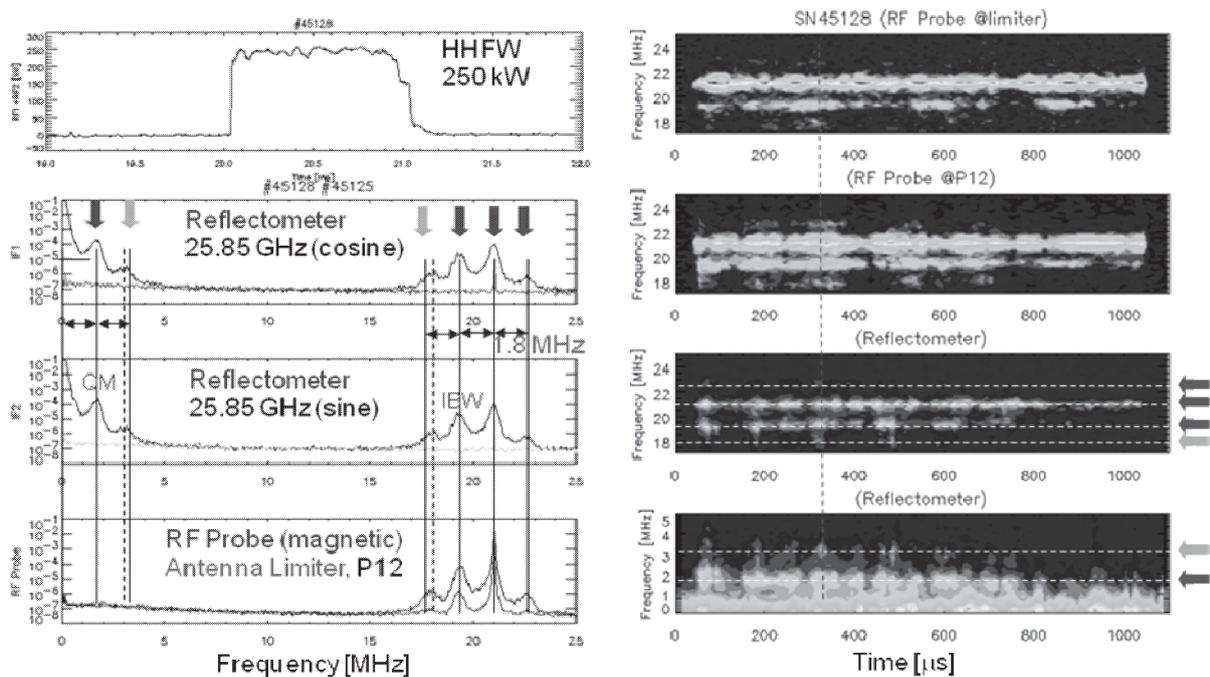
Fig. 1. Detection of the HHFW in the plasma by a reflectometer.
