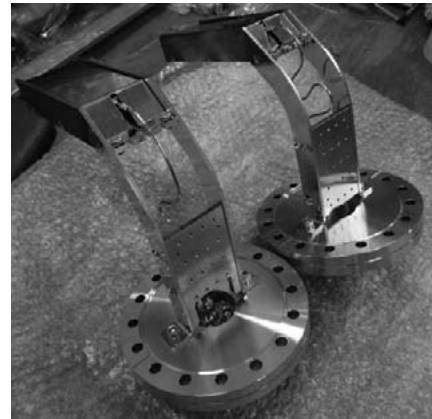
Fig. 1. Newly developed magnetic sensors, BNC type (left front) and multi-pin type (right back)
