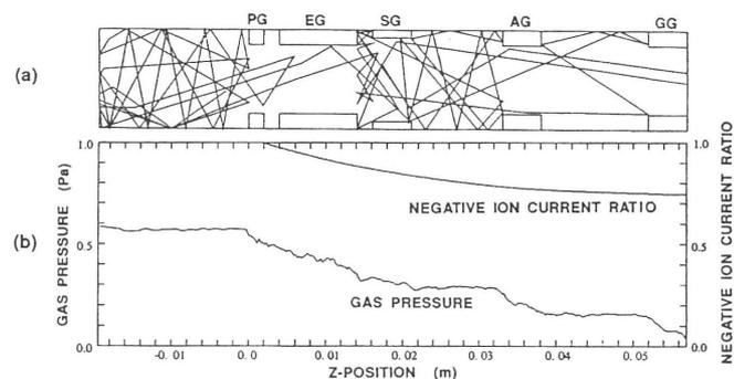
Fig. 1. (a) Example of a gas molecule trajectory, and (b) the gas pressure distribution and the survival negative ion current ratio.
