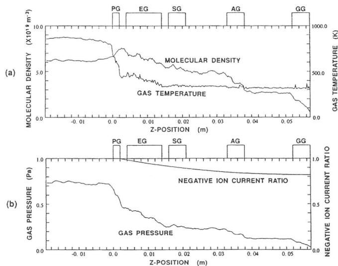
Fig. 2. Results of the Monte-Carlo calculation including gas temperature effect. (a) The gas temperature and the gas molecule density, and (b) the gas pressure distribution and the survival negative ion current ratio.
