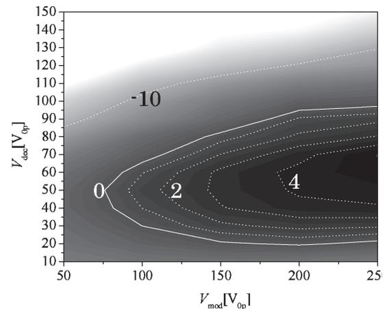
Fig. 3. Calculated Deceleration Efficiency with  $V_n = -2$  kV.
