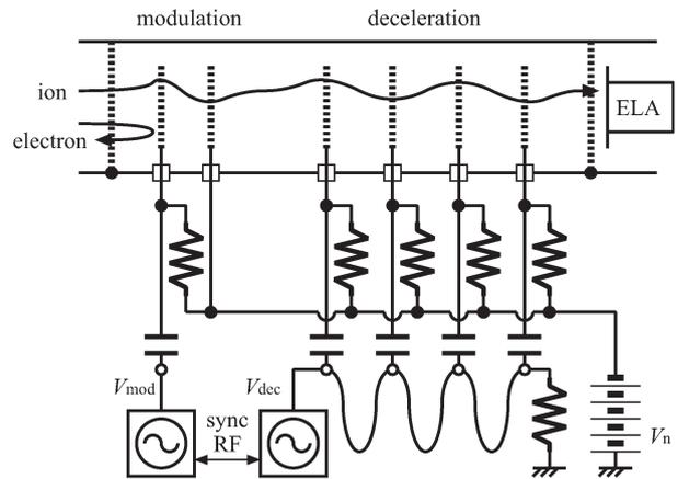
Fig. 1. Schematic diagram of a bias-type TWDEC.
