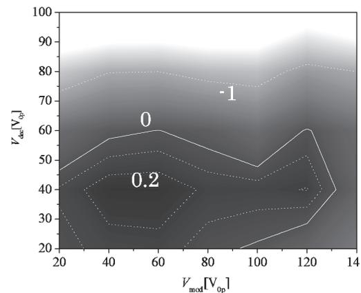
Fig. 2. Calculated Deceleration Efficiency with  $V_n = 0$ .
