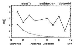
Fig.2 Current characteristics of each antenna element at f = 76 MHz
