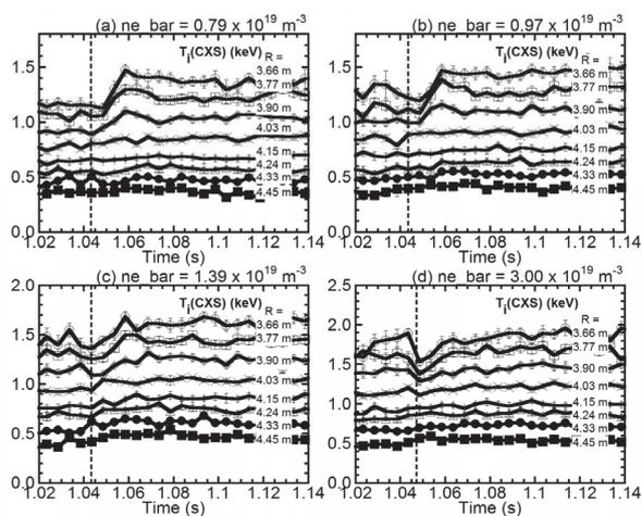
Fig. 2. Dependence of the  $T_i$  behavior in response to the edge perturbation on the line-averaged electron density.  $n_{e, \text{bar}} =$  (a)  $0.79 \times 10^{19} \text{ m}^{-3}$ , (b)  $0.97 \times 10^{19} \text{ m}^{-3}$ , (c)  $1.39 \times 10^{19} \text{ m}^{-3}$  and (d)  $3.00 \times 10^{19} \text{ m}^{-3}$ . Experimental conditions are the same as those of the discharge shown in Fig. 1.
