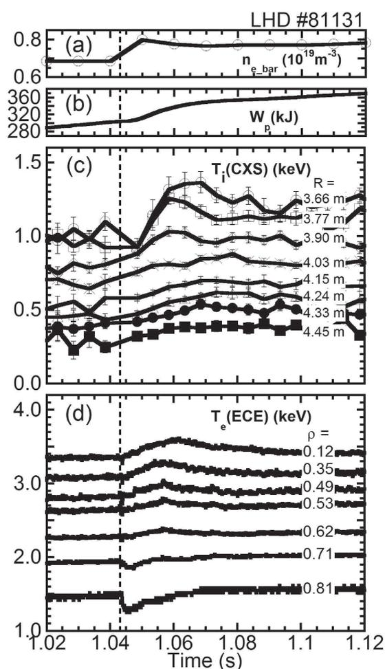
Fig. 1. Temporal evolution of (a) the line-averaged electron density, (b) the plasma stored energy measured by the diamagnetic flux loop, (c) the ion temperature measured using the charge exchange spectroscopy at different major radii and (d) the electron temperature measured with the ECE radiometer at different normalized minor radii. The vertical dashed line represents the time of the TESPEL injection.
