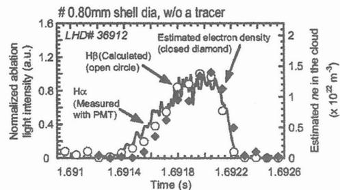
Fig. 2. An example of the temporal evolution of the estimated electron density (closed circle) and the Balmer beta line intensity (closed diamond), which is calculated from the fitted Lorentzian curve, in the TESPEL ablation cloud. The solid line indicates the Balmer alpha line emission from the ablation cloud (solid line) measured with the photo-multiplier.
