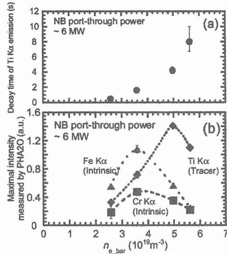
Fig. 1. The dependence of (a) the decay time of Ti K $\alpha$  emission and (b) the maximal intensity of the emissions of Fe K $\alpha$ , Cr K $\alpha$  and Ti K $\alpha$  measured by PHA at Port 2-O on the line-averaged electron.
