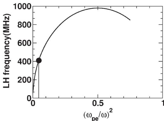
Fig. 1 : LH wave frequency in the pure hydrogen plasma plotted as a function of  $(\omega_{pe}/\omega)^2$  that is proportional to the electron density at the UHR layer. Here,  $\omega_{pe}$  is the plasma angular frequency and  $\omega$  is the wave angular frequency.
