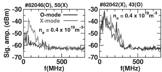
Fig 2. : Frequency spectra in LH wave range of frequency in the case of (a) perpendicular launching for usual ECH, and (b) oblique launching for X-B heating. Sensitivity calibration for each frequency is not done.
