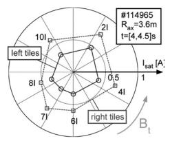
Fig. 2. Toroidal distributions of  $I_{\text{sat}}$  measured at left (blue line) and right tiles (green dashed line) during  $R_{\text{ax}} = 3.6 \text{m}$  discharge with reversed  $B_{\text{t}}$ .
