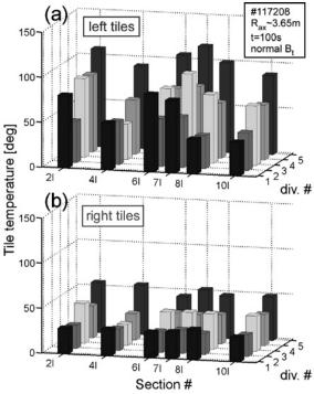
Fig. 3. Tile temperatures measured at (a) left and (b) right tiles at t = 100 s in a steady state discharge.
