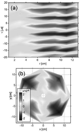
Fig. 1. (a) Cross-correlation function of floating potential at the target plate and band-passed plasma potential measured with GNBP as functions of r and  $\tau$ . (b) Converted image of the cross-correlation by using Eq. (1).
