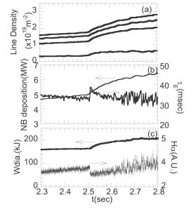
Fig.1 Time trace of (a) line density (from upper, chord position at the equatorial plane is  $\rho = 0.34, 0.58, 0.81, 1.05$ ) (b) Deposition power and  $\tau_E$  and (c) Stored energy and  $H\alpha$
