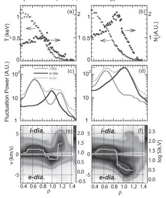
Fig.2 Comparison of profiles before and after transition. (a), (b)  $T_c$  and  $n_c$  profiles (c), (d) spatial profile of fluctuation power spectrum and (e), (f) spatial profile of poloidal phase velocity. (a) is at t=2.3 sec, (c) and (e) are at t=2.3~2.35sec. (b), (b) is at t=2.7 sec, (d) and (f) are at t=2.7~2.75sec.
