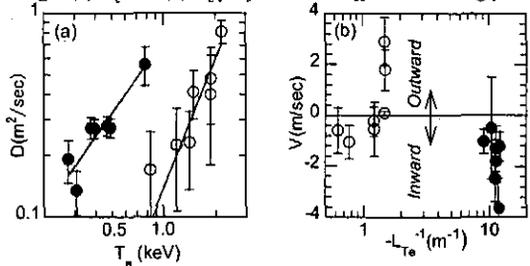
Fig.2 (a)  $T_e$  dependence of D (b)  $-L_{Te}^{-1}$  dependence of V.  $\circ$  and  $\bullet$  indicate core and edge values respectively.
