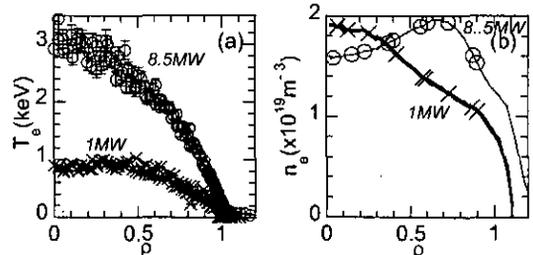
Fig.1 (a)  $T_e$  and (b)  $n_e$  profile under different heating power
