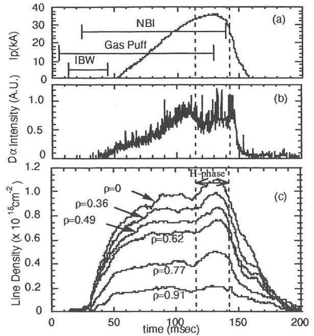
Fig. 1. Temporal evolutions of (a) the plasma current, (b) the  $D\alpha$  intensity and (c) the line density .
