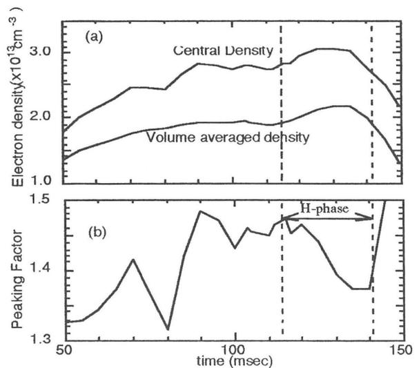
Fig. 2. Temporal evolutions of (a) the central density and the volume averaged density, (b) the peaking factor.
