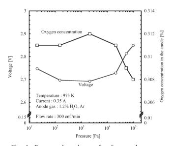
Fig. 1: Pressure dependence of voltage and oxygen concentration in the anode component at 0.35, 973K
