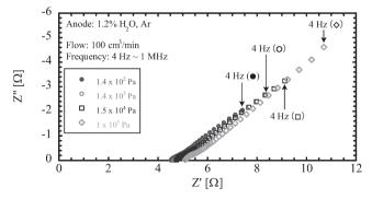
Fig. 2: Pressure dependence of complex impedance measurement in a frequency range of 4 Hz to 1 MHz at  $973 \, \mathrm{K}$
