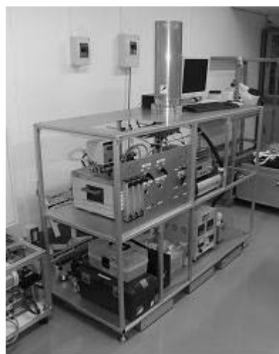
Fig. 2. A photograph of hydrogen isotope pumping system in HRC, Univ. of Toyama.
