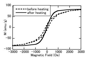
Fig.3 he hysteresis loop of the magnetite sintered by using magnetic field of microwave at 1000 °C.
