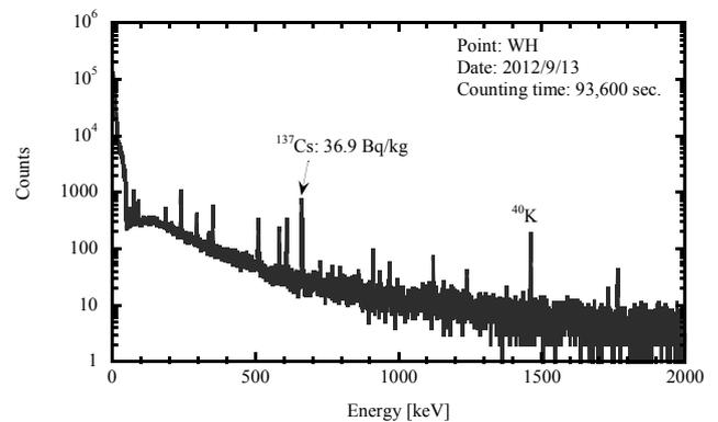
Fig. 1. An example of the measured spectrum of the soil sample by a high purity Ge semiconductor detector
