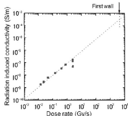
Fig. 3 Dose rate dependence of radiation induced conductivity (RIC) of high purity SiC plate.
