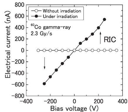
Fig. 2 Example of I-V (current-voltage) curves of high purity SiC plate.
