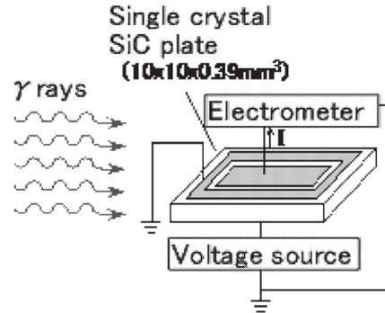
Fig. 1 Schematic drawing of electrical conductivity measurement of high purity single crystal SiC plate.
