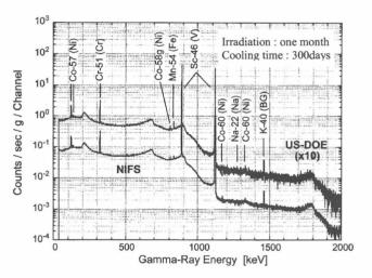
Fig. 1. Example of gamma-ray spectra of vanadium alloy specimens measured 300 days after one-month irradiation.
