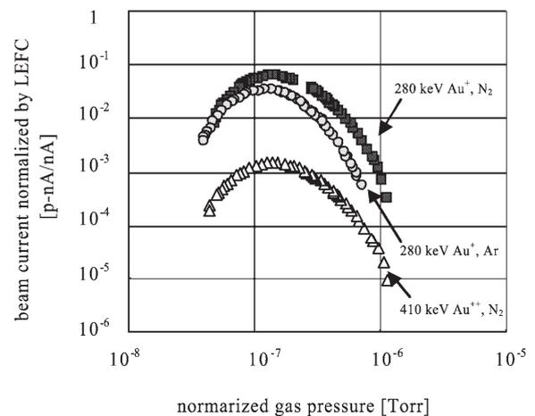
Fig. 1. Ion beam current dependence on gas pressure.
