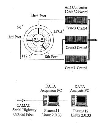
Fig.1 Schematic diagram of three-toroidal-location SXCT system
