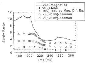
Fig.3 Time evolution of q-values at each minor radius obtained by various methods.
