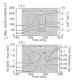
Fig.1 Time evolution of the NBI heated current ramp-up discharge: (a) plasma current, line averaged density and  $H\alpha/D\alpha$  light, (b) ECE signals at the plasma center and the plasma periphery, and soft X-ray emission at the center.
