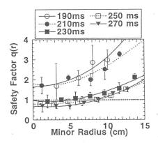
Fig.2 Time evolution of q-profiles obtained by the MSE polarimeter, where the profile is obtained for 20 ms for the marked mean time.
