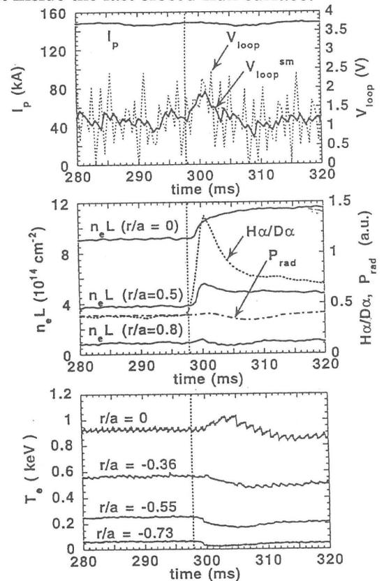
Fig.2 Time evolution of the ohmic plasma when a small ice pellet is injected. (Upper figure) plasma current, loop voltage and smoothed one, (Middle figure) line integrated electron density,  $H\alpha/D\alpha$  light and total radiation power, and (Lower figure) electron temperature obtained by ECE .
