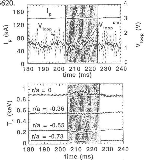
Fig.1 Time behavior of the ohmic discharge when the positive bias is applied to the electrode inserted just inside the last closed flux surface.
