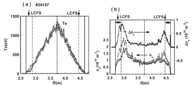
Fig.1 (a) Radial profiles of electron temperature just before (open circle) and after (solid circle) the L-H transition in the configuration of  $R_{\text{ax}}=3.6\text{m}$  and  $\gamma=1.22$  at  $B_t=0.75\text{T}$ . (b) Change of electron density profile and radial profile of the increment of electron density  $\Delta n_e$  across the transition.
