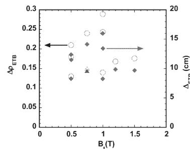
Fig.2 Dependence of ETB width on the toroidal field strength. Solid and open symbols respectively indicate the ETB width  $\Delta_{\text{ETB}}$  and the width normalized by the averaged minor plasma radius  $\Delta\rho_{\text{ETB}}$ . Triangles correspond to the width derived from electron temperature profile and the others from electron density profile.
