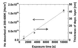
Fig. 1. The relationship between the thickness of the mixedmaterial deposition layer and the areal density of helium desorbed at 300-600 K as a function of an exposure time of the SUS316L specimens to the long pulse discharges
