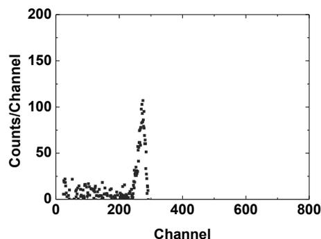
Fig. 2. ERD depth profile of W exposed to the 9th cycle in QUEST
