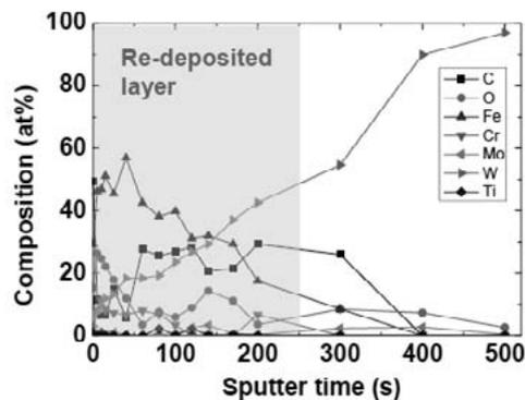
Fig. 1. Depth profiles of surface composition of W exposed to the 9th cycle in QUEST.
