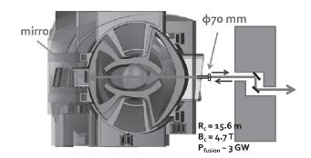
Fig. 1. Example of accessibility for microwave diagnostics in future fusion reactor (FFHR-d1).
