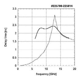
Fig. 3. Observed delay time as a function of launching frequency (solid line) and estimated one (dotted line).
