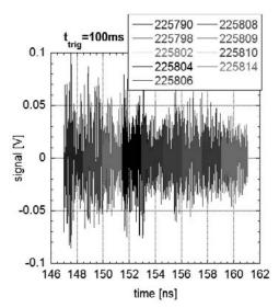
Fig. 2. Temporal waveform of chirping pulsed microwave. Data chain is obtained by some discharges.
