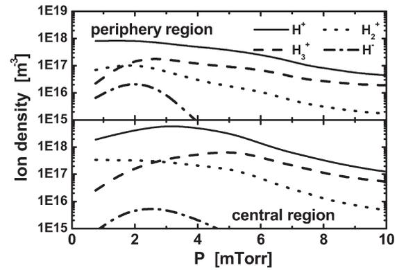
Fig.1 Characteristics of the calculated ion densities ( $H^+$ ,  $H_2^+$ ,  $H_3^+$  and  $H^-$ ) in the periphery region and central region are plotted against gas pressure P.
