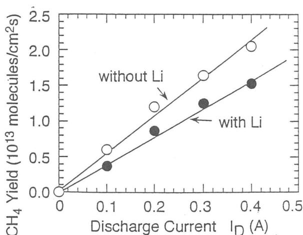
Fig. 1. Discharge current dependence of the CH<sub>4</sub> yield with (filled circles) and without (open circles) the lithium deposition on the graphite wall.
