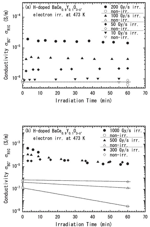
Fig. 1. Radiation induced conductivity,  $\sigma_{\text{RIC}}$ , of H-doped  $\text{BaCe}_{0.9}\text{Y}_{0.1}\text{O}_{3-\delta}$  as a function of electron irradiation time at temperature of 473 K and ionizing dose rates of (a) 10-200 and (b) 300-1000 Gy/s, as compared with base conductivity,  $\sigma_{\text{BC}}$ , before and after irradiation.
