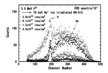
Fig. 2. Typical ERD spectra of helium and hydrogen recoiled from 6H-SiC samples after 10 keV He<sup>+</sup> ion irradiation at several fluences of  $4.0 \times 10^{16}$ ,  $1.2 \times 10^{17}$ ,  $6.1 \times 10^{17}$ , and  $2.8 \times 10^{18}$  ions/cm<sup>2</sup> and room temperature.
