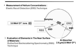
Fig. 1. Schematic view of ion beam analysis systems for helium and hydrogen retained in the SiC materials.
