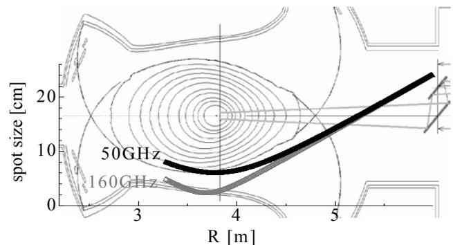
Fig.2 spot size of 50GHz and 160GHz Gaussian Beam.
