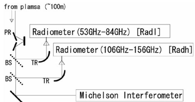
Fig.3 Schematic diagram of the ECE diagnostic system. Each component is connected by corrugated waveguide. PR: polarization rotator, BS: beam splitter, TR: transition from corrugated waveguide to WR12 rectangular waveguide
