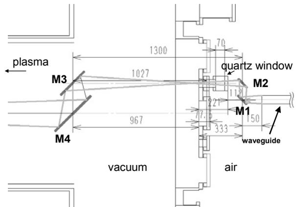
Fig.1 The layout of ECE antenna system
