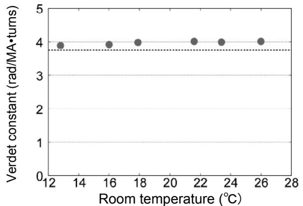
Fig. 3 The Verdet constant of the single-mode flint glass fiber evaluated as a function of the room temperature. The horizontal line indicates the catalog value at 1550 nm.
