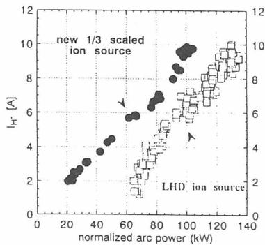
Fig. 1. Arc dependence of  $H^-$  currents in a new 1/3 scaled ion source (close circles) with that of a source for LHD-BL1 (open square).
