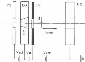
Fig. 2. Assembly of electrodes for a new ion source.
