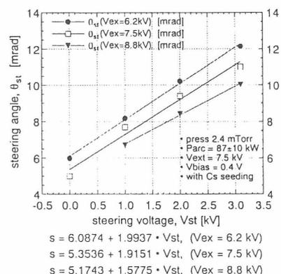
Fig. 3. Beam steering angle by applying voltage to steering electrode.
