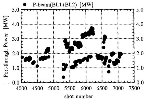
Fig. 2. The sum of port-through powers injected by NBI beam lines numbered 1 and numbered 2.
