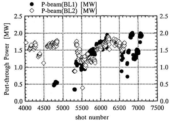
Fig. 1. Individual port-through powers injected by NBI beam lines numbered 1 (closed circles) and numbered 2 (open diamonds).
