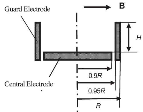
Fig. 1 Schematic drawing of ion sensitive probe.
