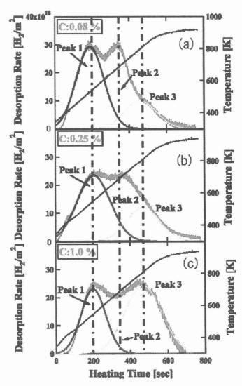
Fig.1 TDS spectra from boron thin films irradiated by 1 keV H<sub>3</sub><sup>+</sup> ion beam. Carbon concentration is 0.08 % for (a), 0.25 % for (b), and 1.0 % for (c). Expermental data are fitted with the sum of three Gaussians (Peak 1, Peak 2, and Peak 3).
