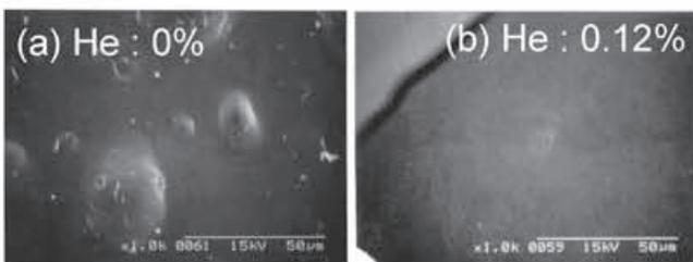
Fig. 1 Blistering due to hydrogen and carbon mixed ion beam irradiation (1 keV  $H_3^+$  as main component, C concentration ~0.8%). Sample temperature is 653 K. Sample is sintered tungsten plate with hot rolled process with stress relieved annealing process.
