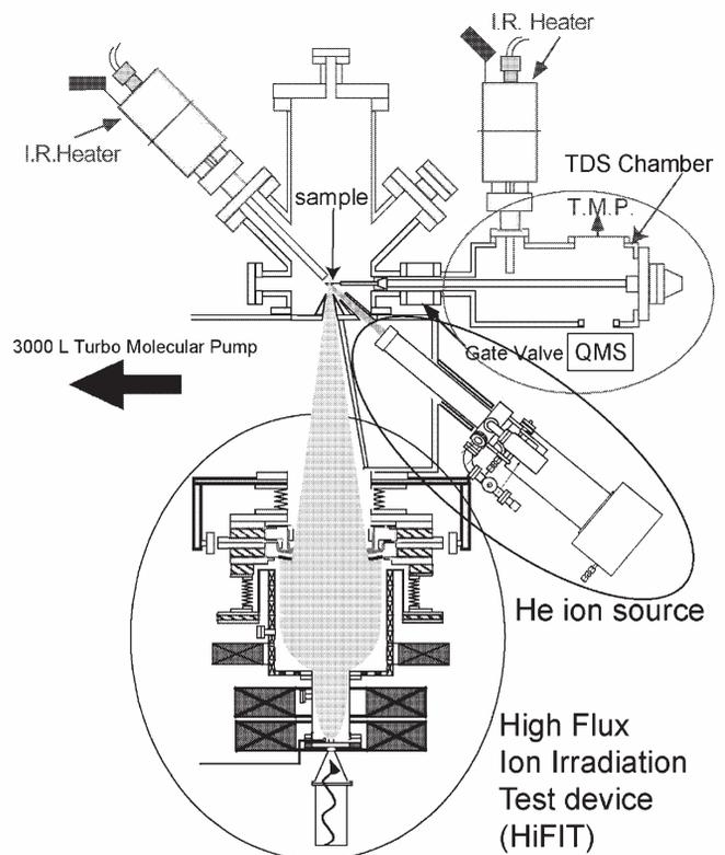
Fig. 2 New H and He ion beam irradiation device
