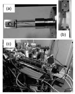
Fig. 1 New sample holders. (a) low temperatures (<500 K) and (b) high temperatures (up to about 1000 K). (c) Linear drive mechanism of the holders.
